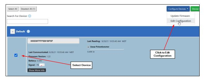
In the dialog box that appears, scroll down to the **Sensor Options** section to find configuration options for the **Potentiometer Sensor** as pictured here:
