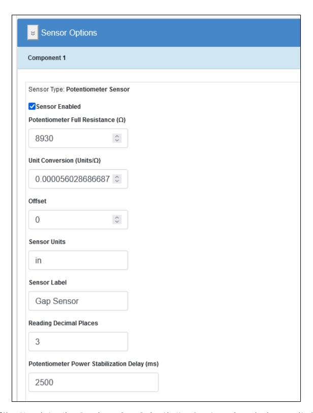
If Phase IV sent the **Leap Linear Potentiometer Sensor Device** with a Linear Potentiometer Sensor already connected it will already be configured and calibrated. Adjusting the configuration won't be necessary. If connecting a Linear Potentiometer Sensor in the field adjust the options as appropriate as described below:
