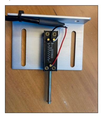
Important: To ensure the most accurate readings solder all wire connections with quality solder joints. Insulate connections at the joints to prevent any shorts.
