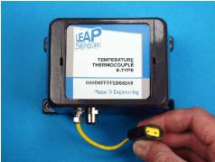
The proper type connector and proper thermocouple wire must be used to accurately measure the temperature at the probe tip.
