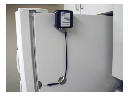
Extra cable may be folded-up and attached to the side of the refrigerator with foil stickers. It will not harm the thin cable to fold it.
