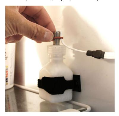
Use the special cold-temperature foil stickers to route the cable out of the refrigerator.
