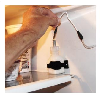
Place the o-ring over the wire to keep the wire from pulling the probe out of the jar.
