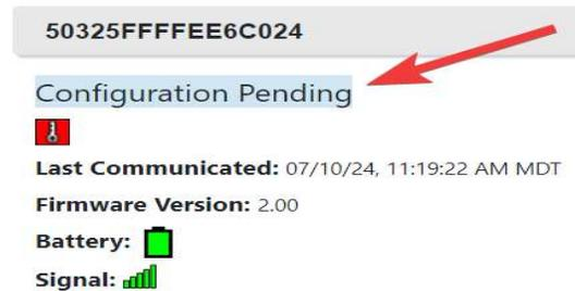
**Figure 12: "Configuration Pending" message appears after changes pushed to the Sensor**
