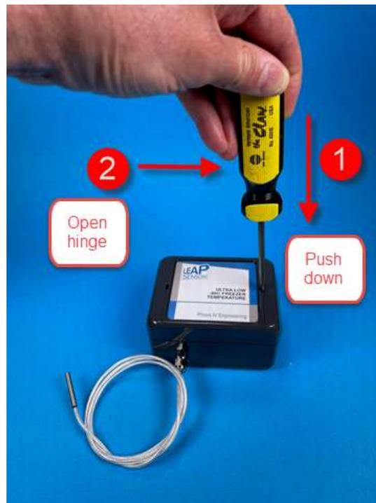
**Figure 40: Opening the Enclosure For Battery Replacement**
