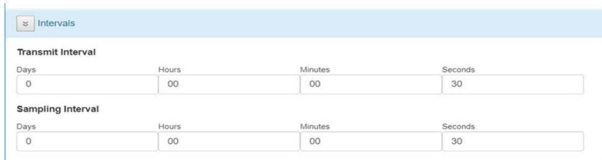
**Figure 11: The "Device Timing Intervals" section of our Device Settings. Allows you to configure how often the Sensor takes new samples and transmits them back to the Gateway**
