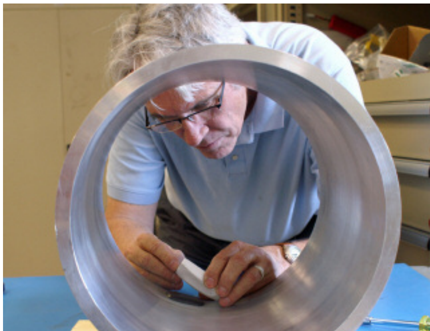
Phase IV engineer Bill Simms spent several weeks developing the right technique for installing RFID sensor tags on the Distillation Assembly's inner drum.
