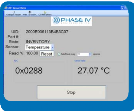
Software Interface for passive SensTAG RFID Temperature Sensor.
