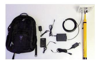
To read the tags, Phase IV designed a kit that includes a backpack with a ThingMagic RFID reader and an antenna with a yellow telescoping handle that ensures users can reach the tags embedded in difficult-to-access liner segments.
