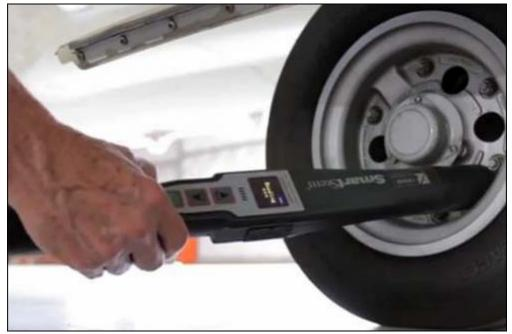
A user places the SmartStem handheld <u>reader</u> over the pressure gauge, which transmits the tire's temperature, pressure and unique ID number.
