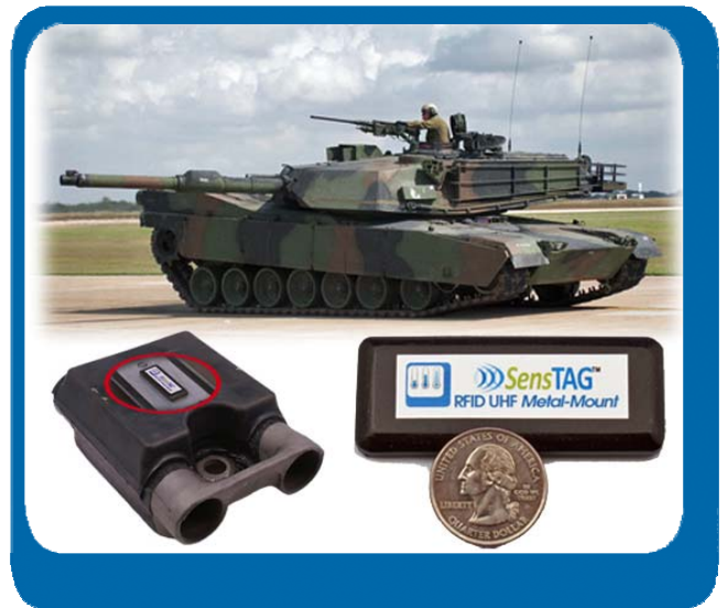
Metal Mounted SensTAGs were embedded in the rubber pads of tank tracks for temperature testing.
