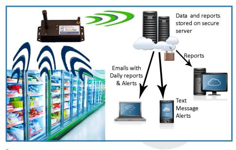
$f^*$  Wireless Sensor and data logger is highly configurable—contact us with your specific requirements.
