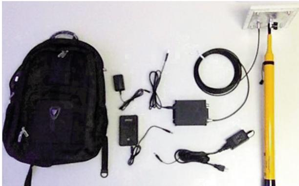
To read the tags, Phase IV designed a kit that includes a backpack with a ThingMagic RFID reader and an antenna with a yellow telescoping handle that ensures users can reach the tags embedded in difficult-to-access liner segments.
