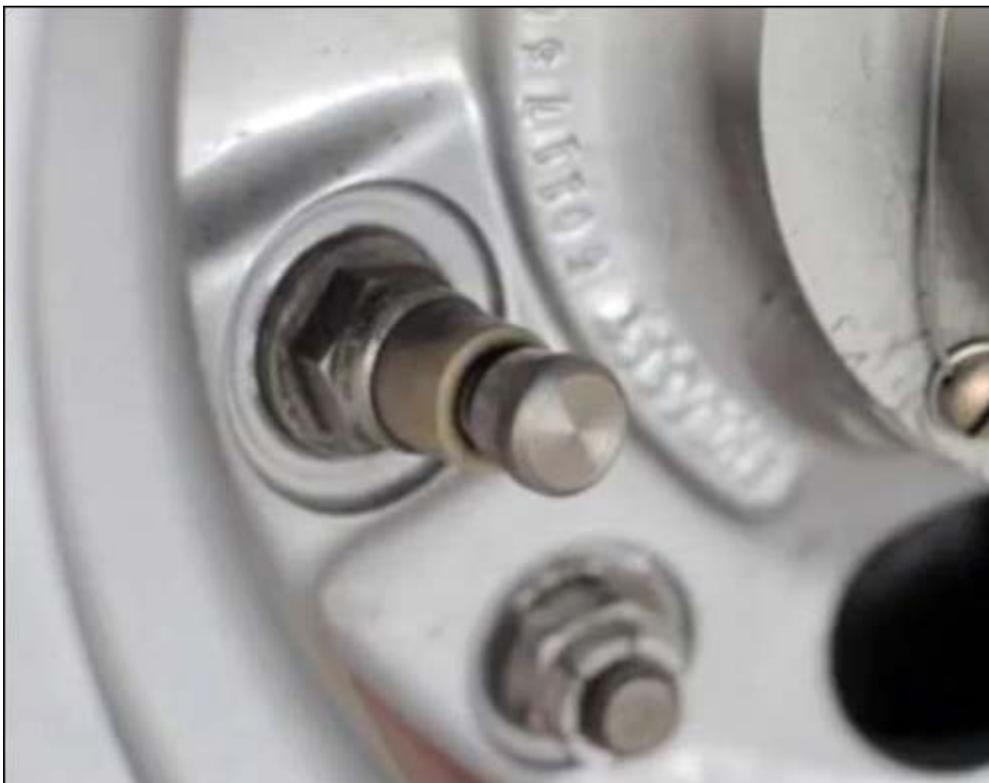
*Crane's SmartStem [RFID](#) air-pressure [sensor](#) replaces a tire's standard fill valve.*
