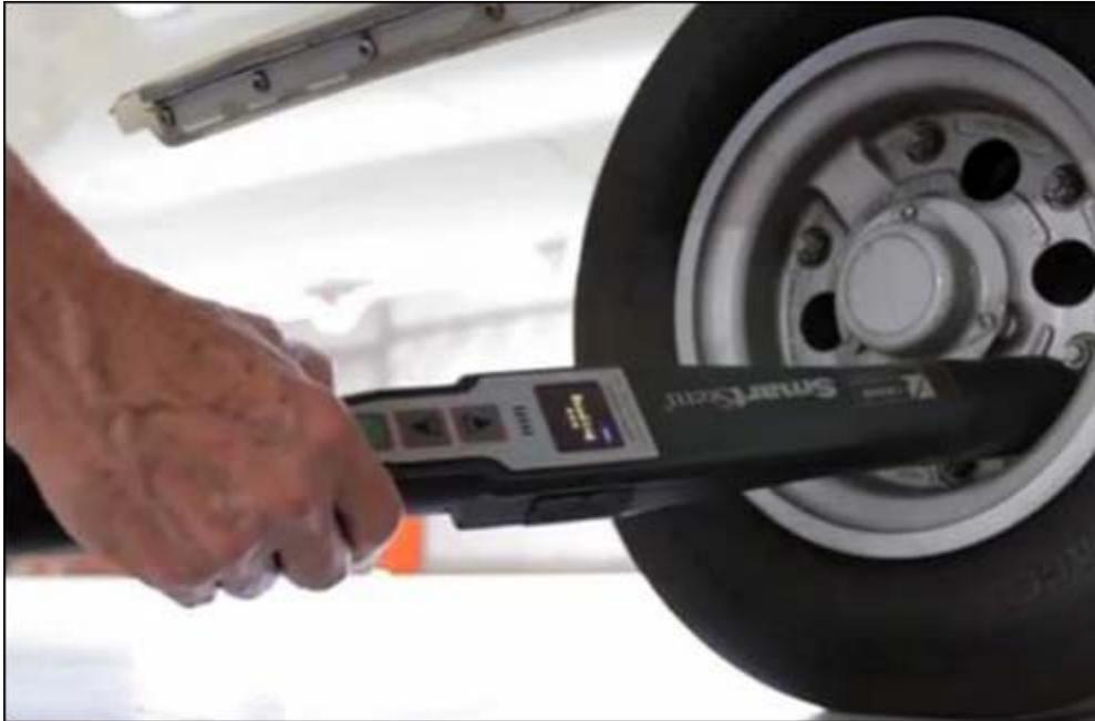
*A user places the SmartStem handheld [reader](#) over the pressure gauge, which transmits the tire's temperature, pressure and unique ID number.*
